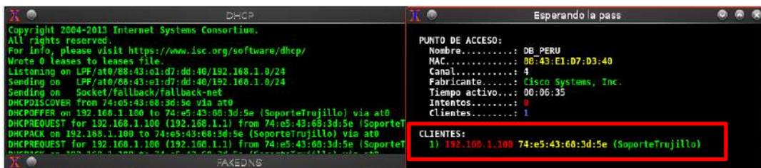
The image shows two terminal windows. The left window displays DHCP logs, including the IP address 192.168.1.100 assigned to the victim. The right window, titled 'Esperando la pass', shows the details of the captured Wi-Fi network, including the SSID 'DB\_PERU', MAC address '08:43:E1:D7:D3:40', and a list of clients, with the victim's device highlighted in a red box.
