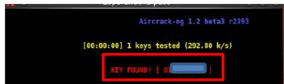
The image shows the Aircrack-ng 1.2 beta3 r2393 interface. It displays the progress of a brute-force attack: '[00:00:00] 1 keys tested (292.80 k/s)'. A red box highlights the message 'KEY FOUND! [ 01: ]', indicating that the correct Wi-Fi password has been discovered.
