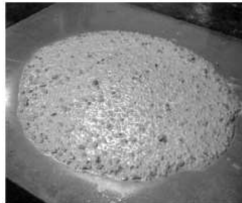
FIG. X1.2 VSI = 1 – Concrete Shows Slight Bleeding Observed as a Sheen on the Surface.
