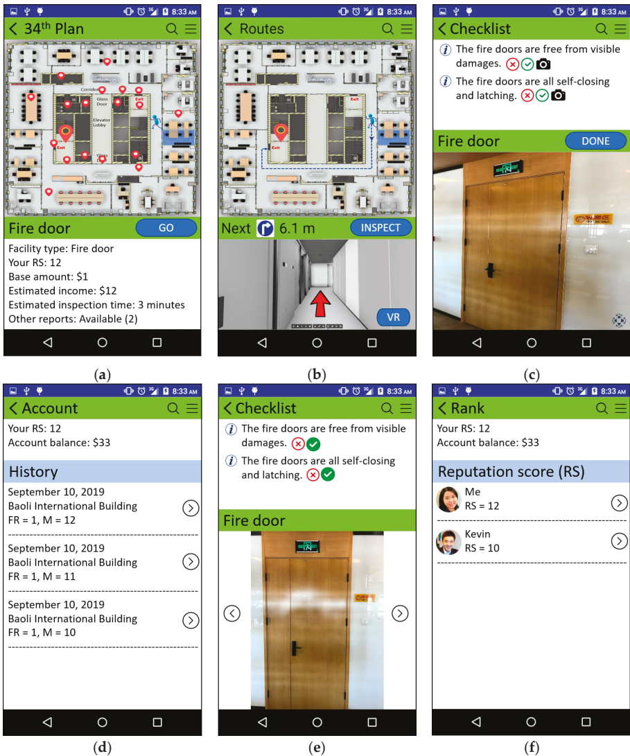
Figure 8. Prototype application of iInspect: (a) Possible inspection locations. (b) Indoor navigation to the inspection location. (c) Items to be inspected. (d) Account overview. (e) Inspection details. (f) Rank details.
