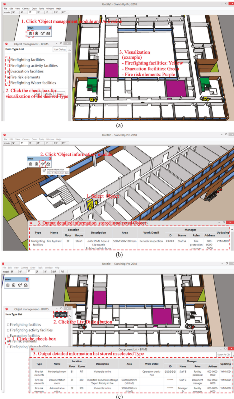
Figure 7. BFIMS implementation: (a) Object visualization; (b) single object data output; and (c) multiple grouped objects data output.
