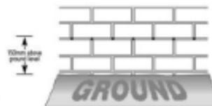
Drilling pattern for Stretching Bond
