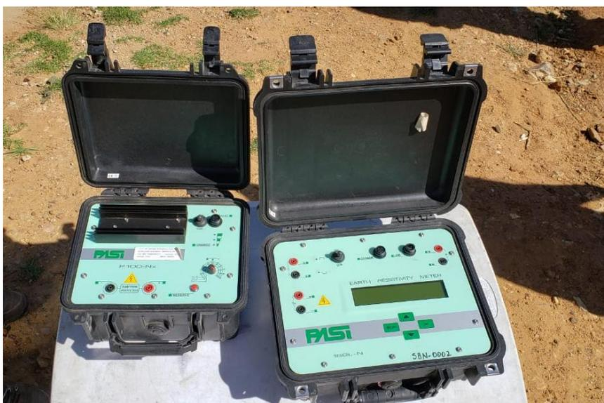
Figura 2. Resistivimetro Transmisor-Receptor, MARCA PASI
