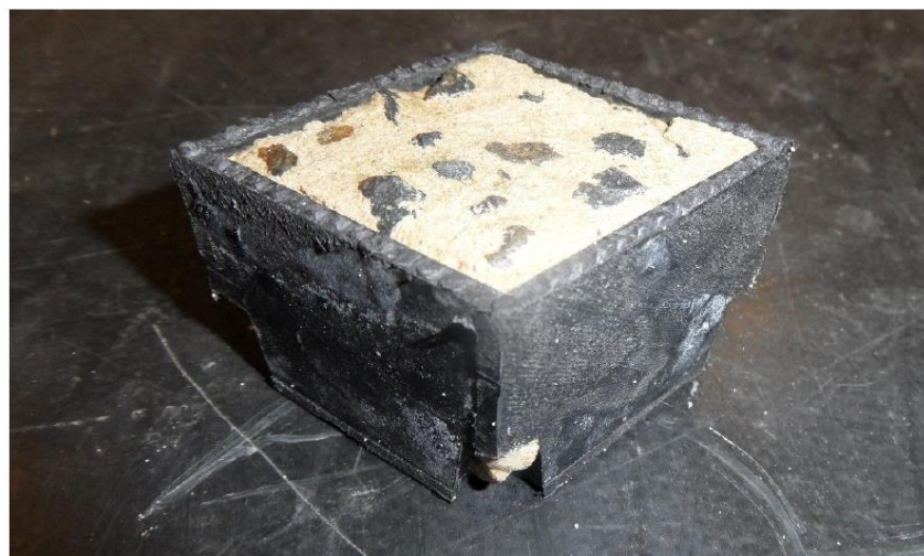
Figure 2: Testing configuration A - a single cell of the grid was extracted and the compression stress of the unit assessed.
