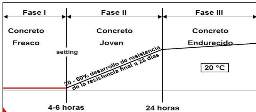
Figura 2. Requisitos ASTM C494
